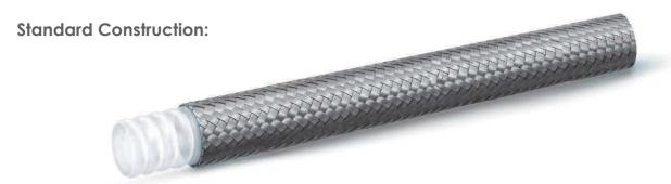
**Inner Tube:** helically Convoluted PTFE tube made of selected premium materials certified in compliance with RoHS Directives and FDA Regulation 21 CFR 177.1550. Advanced processing and quality control ensure best quality, excellent flexibility and kink resistance.
