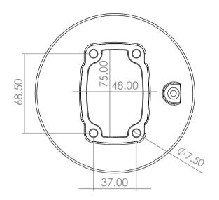
Ø134mm Panel Coupling provides the connection between the operator arm and the operator panel. ARM130.310 is a fixed module. The diameter is 130mm and produced for wide panels with depth.
