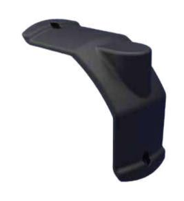
ARM130.810 Warning Lamp Cover (M22) is placed on the corner module ensuring an area for the warning lamp to be placed. The warning lamp connection diameter is M22×1.5
