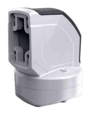
ARM130.550 Rotatable Panel 90° Angle Coupling is suitable for an operator panel that requires positioning directly after a 90° angel corner turn. Max. diameter is 123mm and the rotation angle is 315° in total. The ability to rotate around itself provides flexibility for the operator using the panel in bringing it to a desired position. ARM130.550 is an ideal product that will be used for the panel types with more depth.
