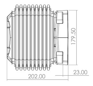
The Steel Wall-Mounted Module - With Bellows helps fixing the operator arms horizontally which are positioned on vertical surfaces. This product with its cast steel body gives reliability for heavy loads and long-distance arm configurations. It allows a mobility of 90° to the right and left.
