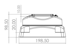
ARM130.610 Rotatable Top Mounted Vertical Outlet provides a 315° rotation movement to the right and left. It is designated for heavy loads configurations and can also serve as a "Fixed Kiosk"
