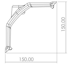
ARM130.811 Warning Lamp Cover (M18) is placed on the corner module ensuring an area for the warning lamp to be placed. The warning lamp connection diameter is M18×1.5 130/080 Support Arm Adaptor is used to secure the connection between ARM130 and ARM080 Its is designed for configurations of heavy loads. The configurations with this product prevent vibrating and sagging as a result of heavy loads. This support Arm Adaptor can be used horizontally or vertically.
