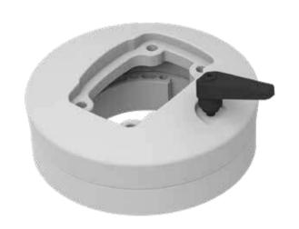
ARM130.320 Rotatable Panel Coupling provides the connection between the operator arm and the operator panel. The diameter is 133mm with a rotation capacity of 315° allowing the operator to rotate the panel to any desired position. It is produced for panel types with high depth ratio.
