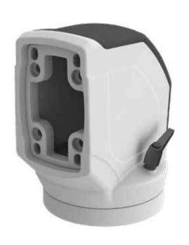
ARM130.400 Rotatable Panel 90° Angle Coupling is suitable for an operator panel that requires positioning directly after a 90° angel corner turn. The rotation angle is 315° in total. The ability to rotate around itself provides flexibility for the operator using the panel in bringing it to a desired position. ARM130.400 is an ideal product that will be used for the panel types with more depth.
