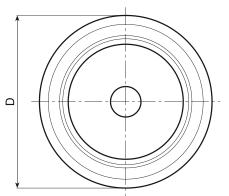
Version with zinc plated insert and H10 tolerance bore
